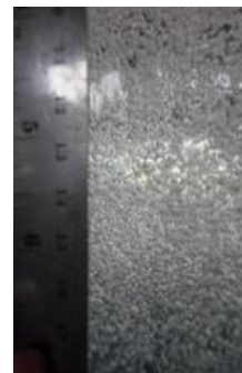
Fig. 6 Photograph of uniform gas bubbly flow.
